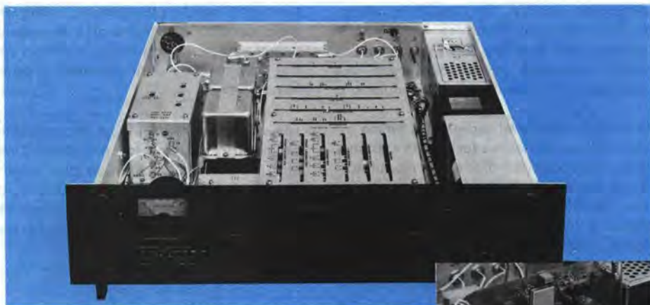
The MCP-1V visual exciter/modulator (one in each of the two 18-kilowatt transmitters included in the BTD-36L2) is a solid-state, independent self-contained "on-channel" signal source. Harris' TSB filter (right) is mounted on a PC board in the visual exciter, and measures only 1 1/2 square inches.
