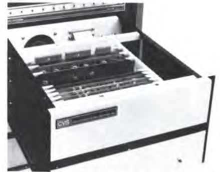
Figure 6: "Slide-out" rack mount chassis provide easy access to all circuitry.
