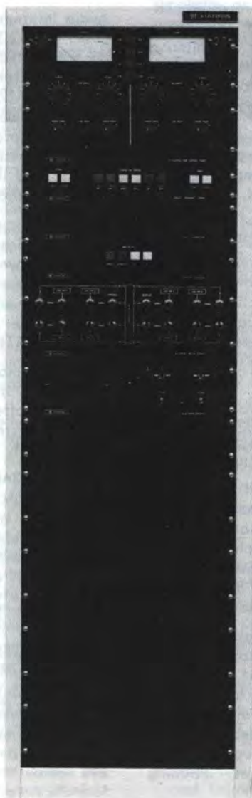
All adjustments for dual transmitter operation may be made from the center control cabinet of the BTD-36L2. An RF Phasing and Control Panel and an Automatic Exciter/Modulator Switcher are standard equipment in the cabinet—and several optional control panels are available.
