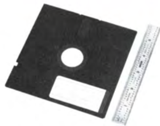
Figure 3: A single, re-usable EPIC mini floppy disc automatically stores 2,000 edits.
